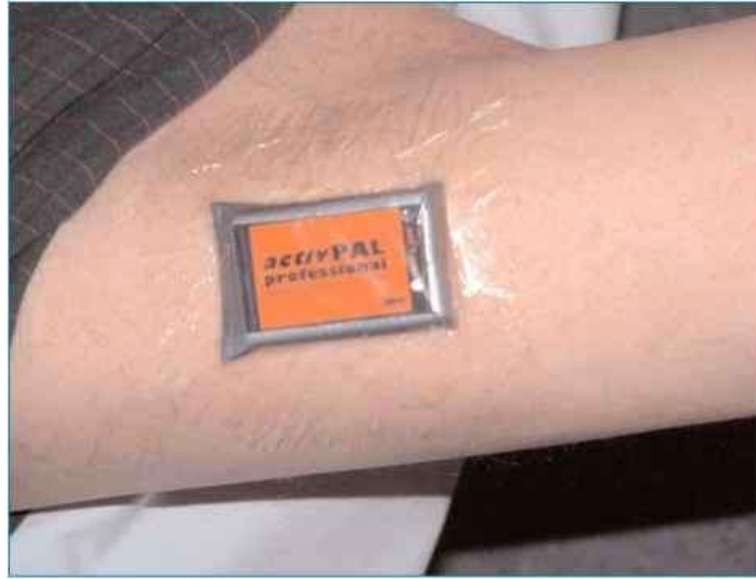
Figure 2.5. activPAL Ambulatory Physical Activity Meter [19]
