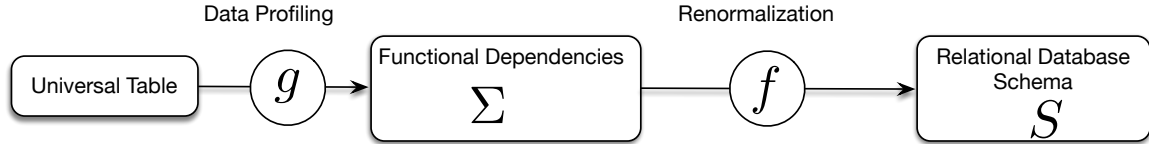
Figure 1.1: The Data flow of generating a database schema from a universal table
