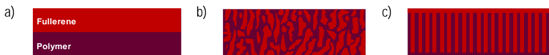
Figure 1.15 Three types of morphologies of the active layer used in polymer solar cells: (a) bilayer, (b) bulk heterojunction (BHJ), and (c) ordered BHJ
