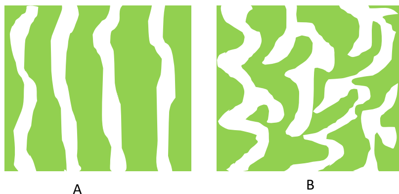
Figure 5.18 Schematically diagram of water permeation pathway on membrane interface (white = aqueous domains), where the pathways of B are less-ordered than in A.
