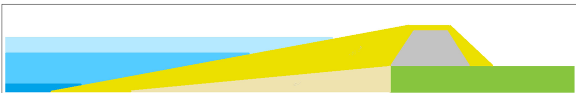
Figure 9. Sand dike with sediment fill
