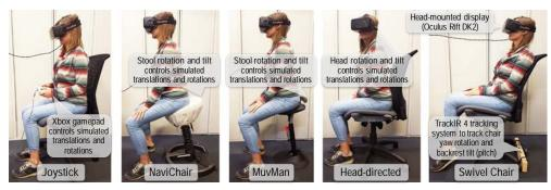
Figure 2: The five interfaces tested in this user study. From left to right: Joystick, NaviChair, MuvMan, Head-Directed, and Swivel Chair.
