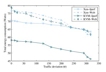
Figure 3.6: Server energy measurements with 8 active VMs
