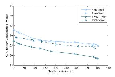
Figure 3.3: CPU energy measurements with 5 active VMs
