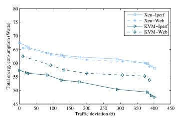
Figure 3.4: Server energy measurements with 5 active VMs
