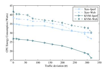
Figure 3.5: CPU energy measurements with 8 active VMs
