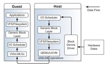
Figure 4.8: KVM disk I/O subsystem
