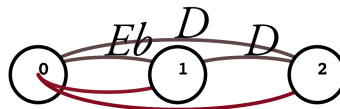
Figure 3.8: Step two: Input ( D ). Add new transitions from state 0 and 1 to state 2 by ( D ) and suffix link to 0.
