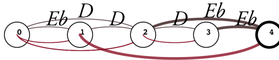
Figure 3.10: Step four: Input (Eb). Add new transitions from state 2 and 3 to state 4 by (D) and (Eb) respectively, suffix link to 1.
