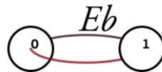
Figure 3.7: Step one: Input ( Eb ). Add a new transition from state 0 to 1 by ( Eb ) and suffix link from state 1 to 0.
