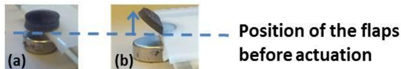
Figure 64: Comparison between the maximum deflections achievable by (a) a 1 mm thick flat-flap actuated under 80 mT external magnetic field; and (b) a 1 mm thick step-shaped flap (similar to the design used in the valve's fabrication) actuated under 80 mT external magnetic field. Diameter of the M-CP flaps = 6 mm. This image is reprinted with permission from [126].
