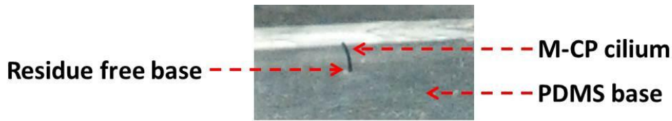
Figure 20: Cilium mixer fabricated by following the extra steps of heating and re-flowing of the PEG sacrificial mold after the insertion of micro-needles. The re-heating and cooling steps ensure that there is no crack or gap between the PEG and the underlying PDMS layer, (cilia diameter = 130 \pm 5 \mu\text{m} , cilia height = 1.2 mm).
