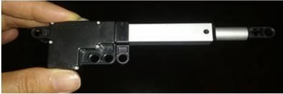
Figure 94: Photograph of the linear actuator, L12-P-50, Fergelli, Inc, used to move the permanent magnet underneath the platform.
