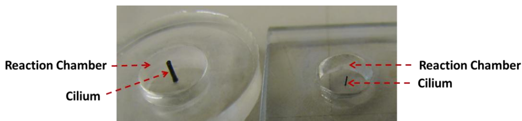
Figure 29: Cilia structures with different diameters fabricated in reaction chambers. (Left) Cilium diameter = 830 \pm 5 \mu\text{m} , (right) cilium diameter = 130 \pm 5 \mu\text{m} .
