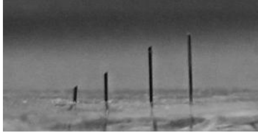
Figure 31: Cilia actuators with different heights fabricated on the same PDMS substrate (cilium diameter for all cilia actuators = 130 \pm 5 \mu\text{m} . Cilium height from left to right: 0.5 \pm 0.1 \text{ mm} , 1 \pm 0.1 \text{ mm} , 1.8 \pm 0.1 \text{ mm} , and 2 \pm 0.1 \text{ mm} ).
