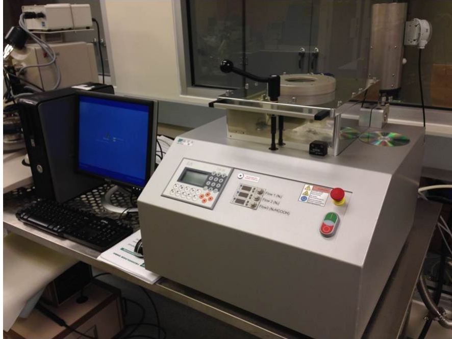
Figure 4.1: Photograph of SRO-700 packaging system
