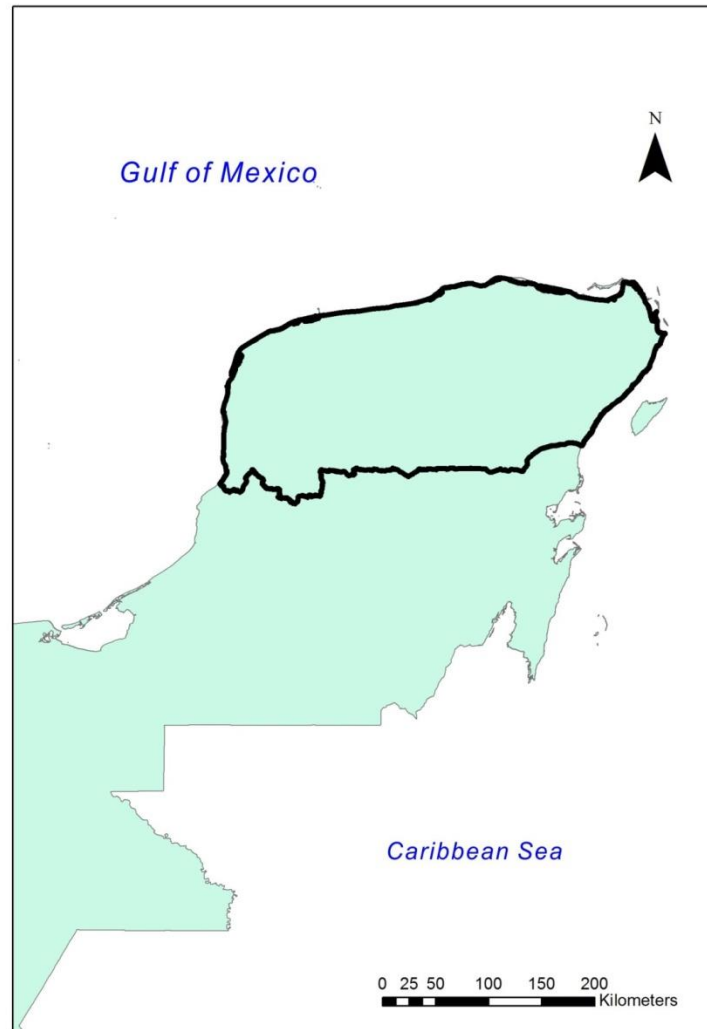
Figure 4.1 The model domain for the Yucatan Peninsula (outlined in black). The coastline of the Yucatan Peninsula was simplified for input into MIKE SHE.
