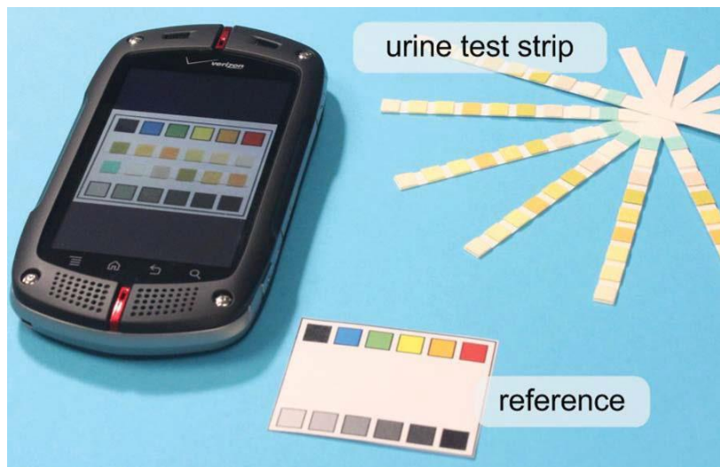
Figure 1.4. Smartphone imaging of commercially available test strips using a color reference chart of known intensities.
