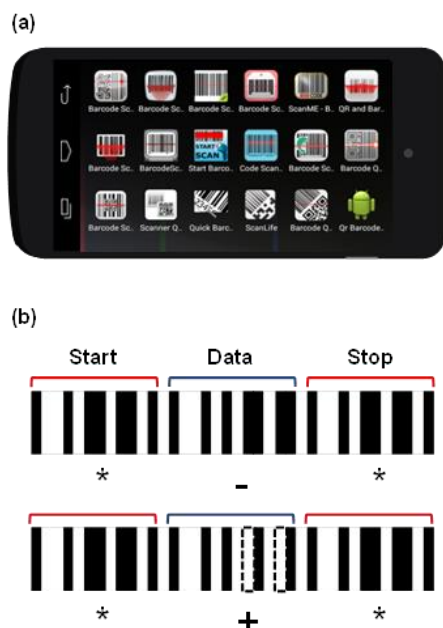
Fig. 2. Barcode scanning apps and barcodes. (a) A set of free barcode scanning apps available for the Android system. (b) Barcodes of the “-” and “+” characters in Code 39. The start and stop character is denoted by “*”. The two data characters are other identical, except for the region highlighted by the dashed lines.
