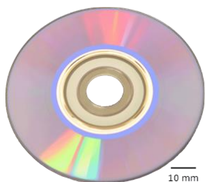
Figure 4.1. Photo of a MiniDVD. It has a diameter of 80 mm and a center hole of 15 mm diameter with a thickness of 1.2 mm.
