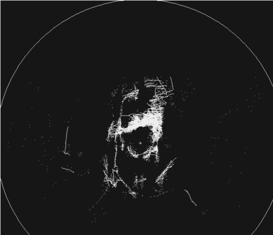
Figure 2.2. Screen capture of the radar imagery video displayed through EchoTrack's processing phase showing radar-defined tracks (white lines) detected during one sampling interval (14 minutes) at one of my sites. The crosshair shows the location of the radar and the circle denotes a 2 km radius.
