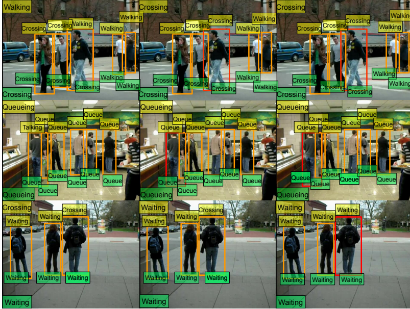
Figure 4.1: Results visualization for our model. Green tags are ground truth, yellow tags are predicted labels. From left to right is without message passing, first step message passing and second step message passing
