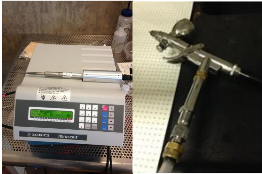
Figure 3-9: The photograph of Ultrasonic Homogenizer and spraying gun
