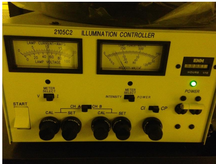
Figure 3-6: The illumination controller and the parameters shown in the meters
