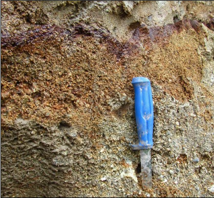
Figure 3-8. The placic horizon is thin, vitreous, and nearly flat, and is located above the top of the knife. Knife handle is 11 cm in length.
