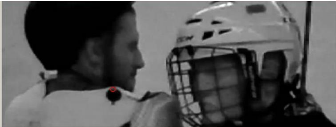
Figure 2.7. Screenshot of a frame from the high-speed camera. The video clip was loaded into the DLTdv5 toolbox that was used to digitize the location of a marker located on the back shoulder of each shoulder pad. The red circle denotes the point marked by the toolbox for this particular frame. A minimum of fifteen frames prior to contact were digitized in order to differentiate the resulting position data into velocity units.
