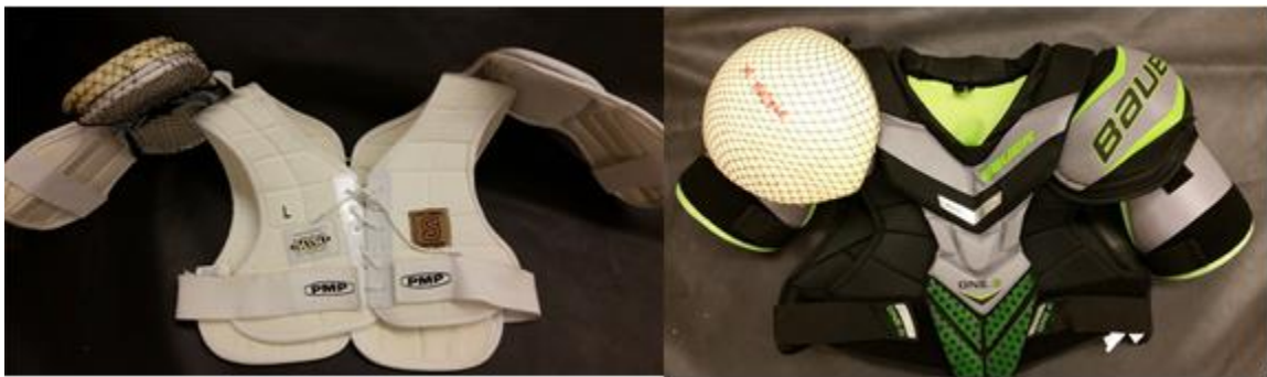
Figure 2.4. Diagram showing Pad A (on left) and Pad B (on right) with the moulded foam cap adhered on top of the right shoulder cap. Pad A is lighter in construction than Pad B and contains much less foam over its plastic cap. Pad B contains multiple layers of foam over its plastic cap and features a more rounded cap profile. The foam overlays that were moulded for each pad were 2cm thick and designed to match the shape and curvature of the underlying plastic cap.
