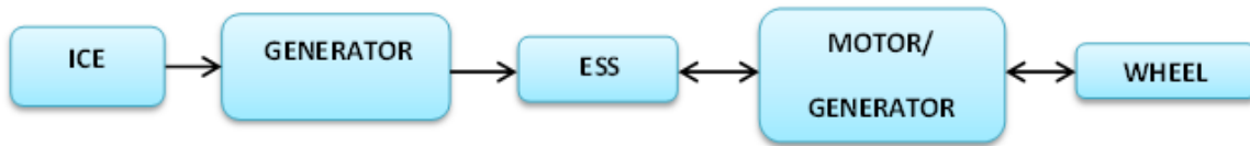
Figure 3-1: Series powertrain configuration, ESS: Energy Storage System
