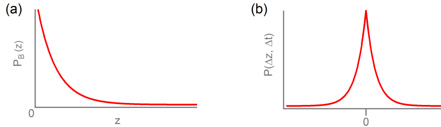
Figure 2.6: (a) Form of the Boltzmann distribution assuming a gravitational potential only. (b) The long-time stationary bi-exponential (Laplace) distribution of displacements.
