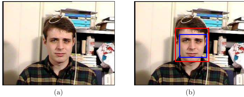
Figure 3.11: (a) a sample frame from Boston University dataset [37], where a person is wearing a 3D magnetic tracker to collect ground truth for head pose; (b) the red rectangle indicating the detected face by Viola-Jones algorithm [65], and the blue rectangle indicating the detected ROI.
