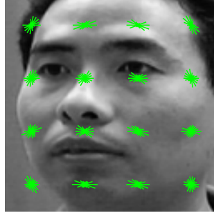
Figure 3.7: Orientation information in HOG. Within the face image from Figure 3.5, green lines indicate orientation generated from gradients. For each cell, there are totally 9 bins for orientation distribution.
