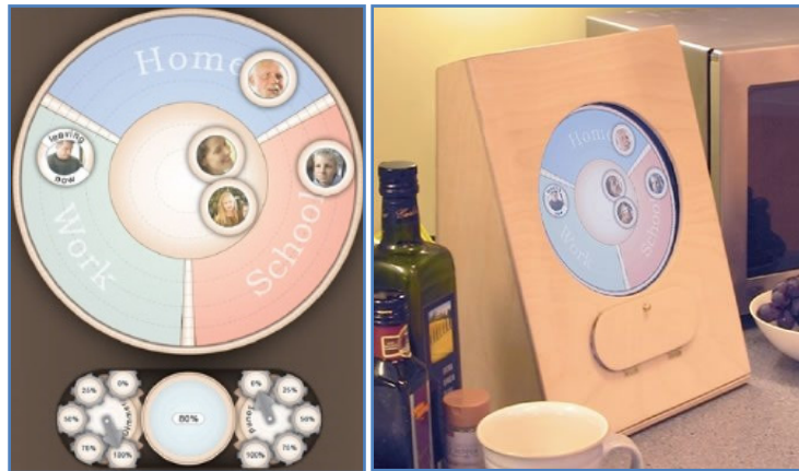
Figure 2.4: The Whereabouts Clock showing family members locations (Left) and placed in the kitchen (Right) (Copied with permission from Sellen et al., 2006)
