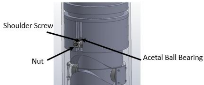
Figure 3-4. Structure of the Side Lock
