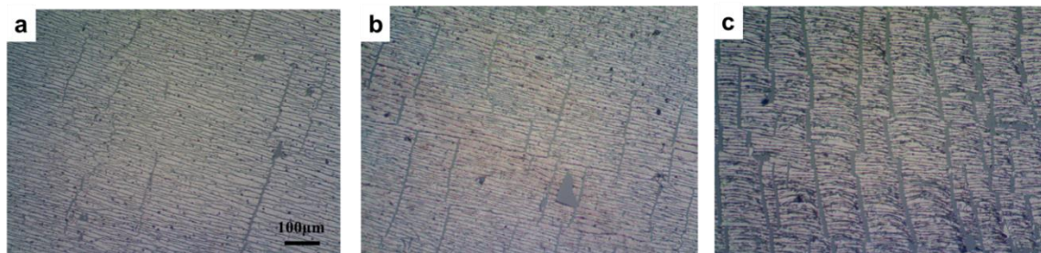
Figure 3.26. Microscopic pictures of r-GO thin films transferred by RPM ratio of (a)1.4, (b)1.6, and (c)1.8. Higher stress induced by higher RPM ratio forms more cracks and wrinkles on the transferred film.
