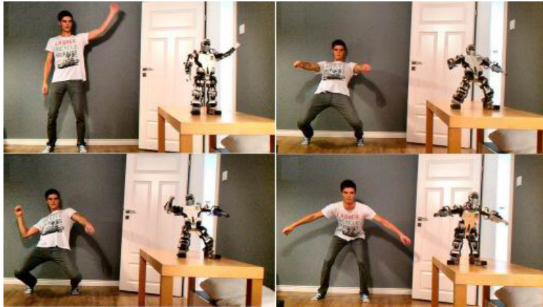
Figure 1.4 Mapping body pose to anthropomorphic robot through the use of Kinect skeleton tracking [4]
