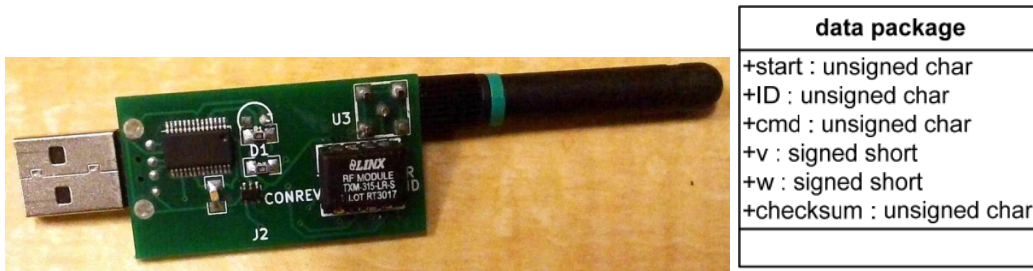
Figure 2.5 (A) USB Transmitter Board (B) Data package [6]
