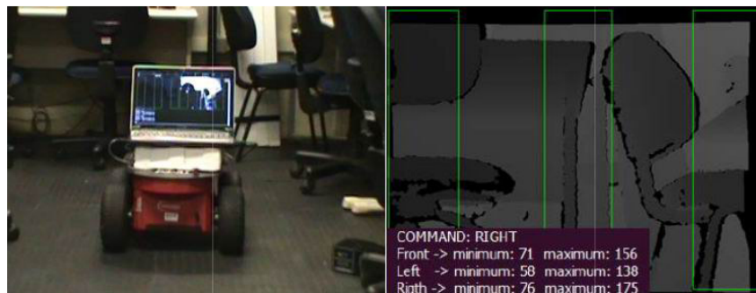
Figure 1.5 (A) Autonomous surveillance robot (B) Depth camera view and decision window [5]
