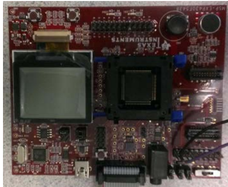
Figure 6.3: The communication unit based on a MSP430 evaluation board.
