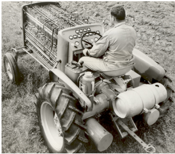
Figure 1.2: Allis-Chambers tractor using 1008 fuel cells for power. (Photo courtesy of Smithsonian Science Service)
