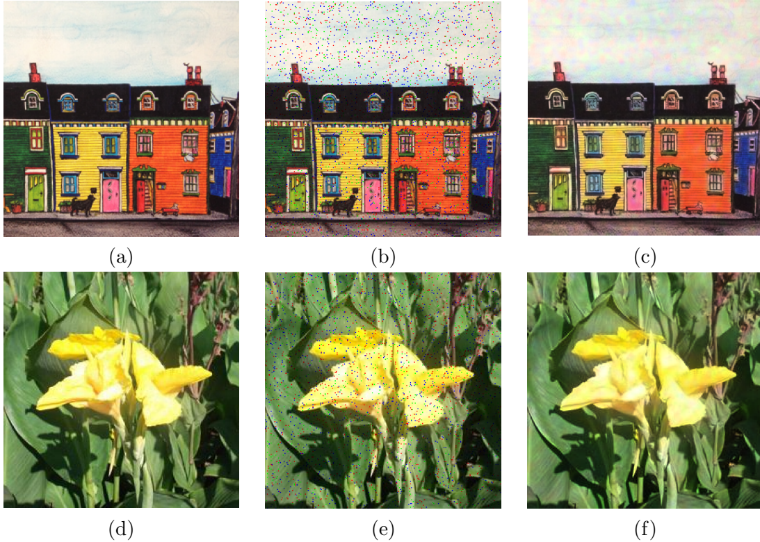
Figure 4.4: Isotropic diffusion of chromaticity noise for two 256 \times 256 pixel images: cartoon of Newfoundland row houses [19] (first row) and natural scene of flowers (second row). The noisy image (b) was denoised to give (c) after 25 time steps. The noisy flower image in (e) took 30 time steps to give the denoised image in (f).
