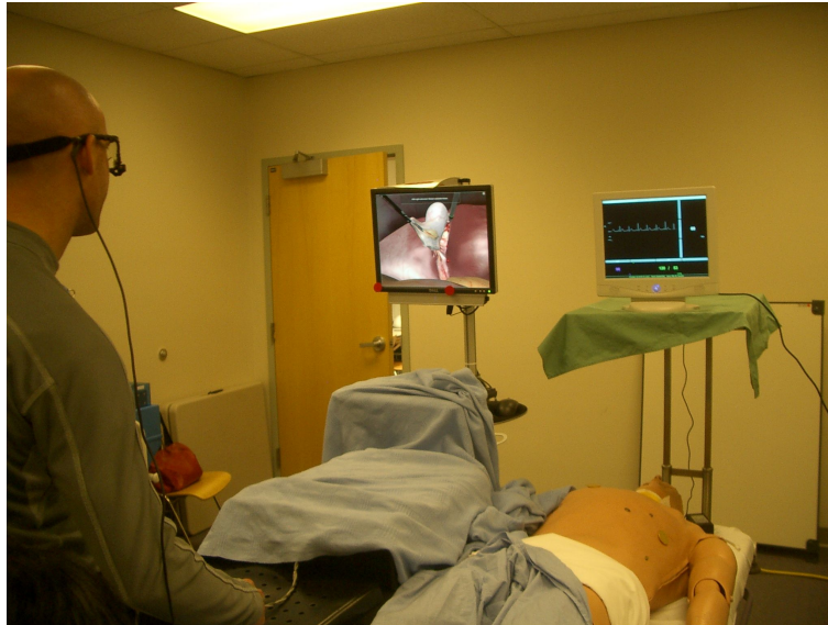
Figure 3.2: A subject being eye tracked with a PT-Mini while operating the SurgicalSim VR with patient vitals displayed using ECS.
