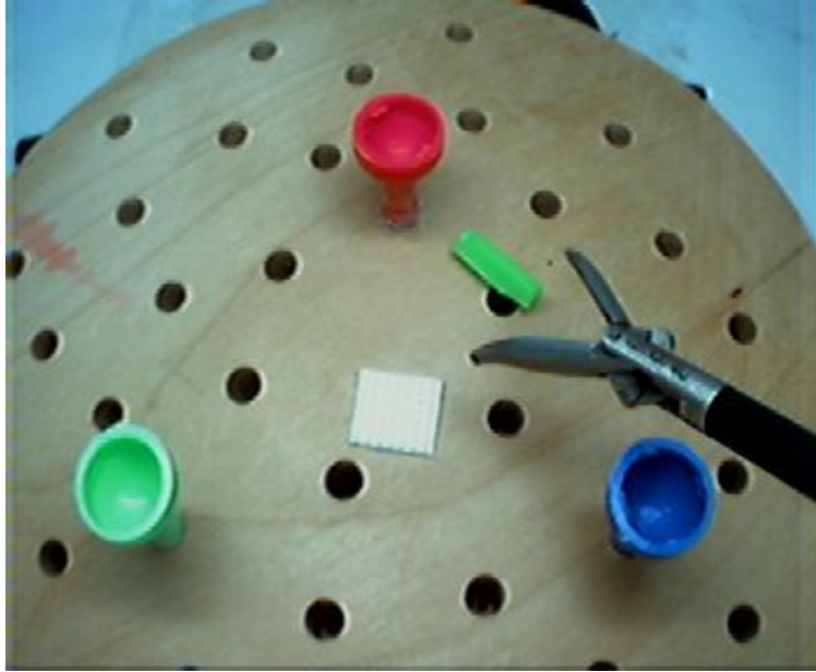
Figure 5.2: Screen capture of the peg transfer physical arrangement. While the physical arrangement is uniform, this view presents a perspective transformation due to the oblique viewing angle of the training box’s fixed internal camera.
