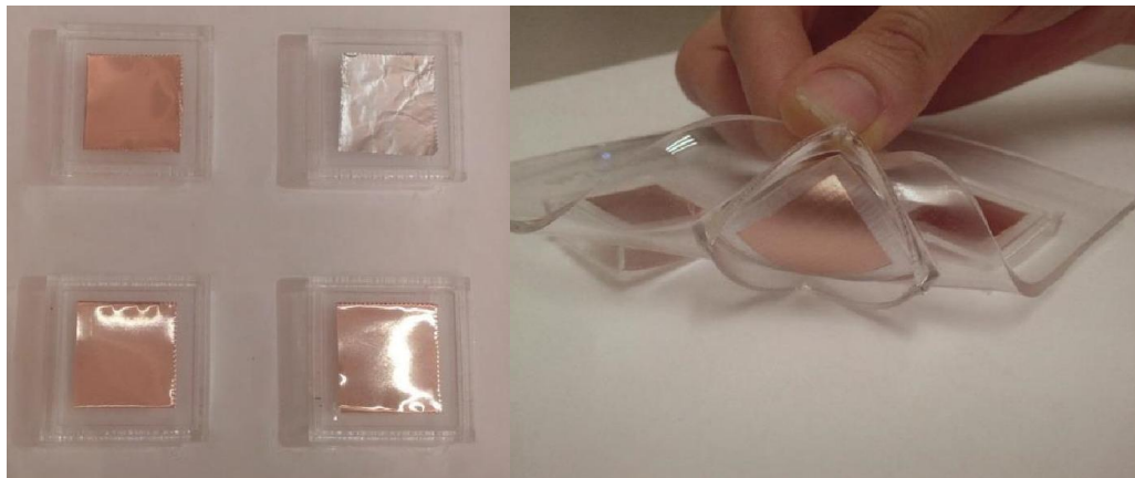
Figure 3.6: Fabricated interface by embedding thin copper (reddish brown color) and aluminum (bright grey color) film in PDMS to create flexible conductive targets.
