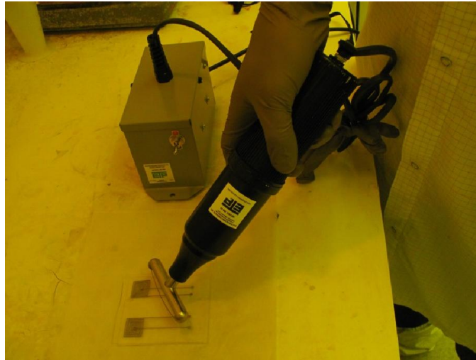
Figure 3.3: Experimental setup for bonding a two-layer PDMS substrate together using the corona surface activation device.
