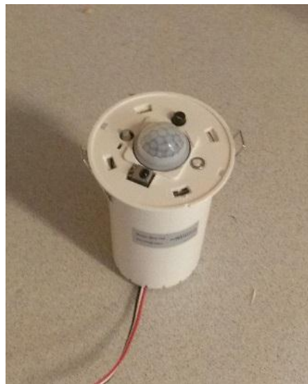
Figure 5.2. Xeleum XCO-100 [45] used as the ambient light sensor in the test bed.
