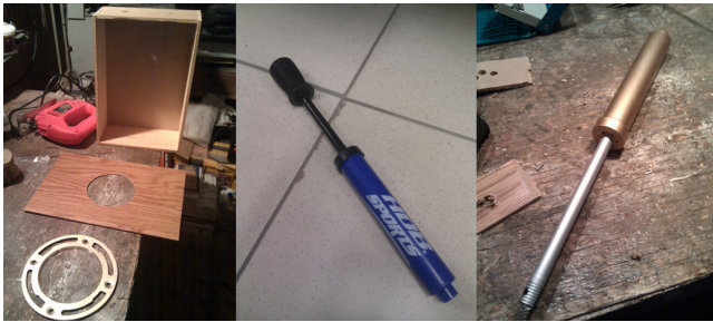
Figure 4. Appropriated basketball pump for a piston.
