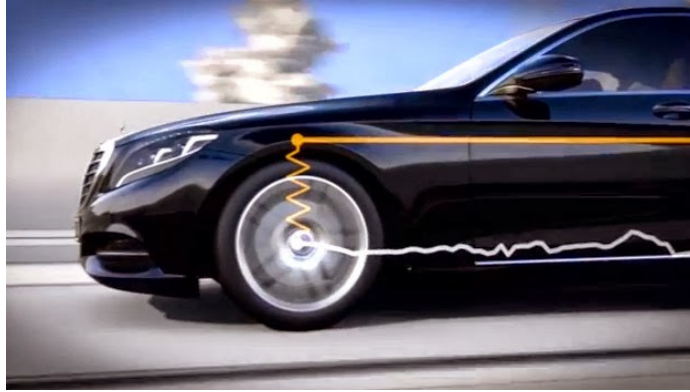
Figure 2-3: Rendition of SDOF Mercedes- Benz S class front suspension under road- excitation [12].
