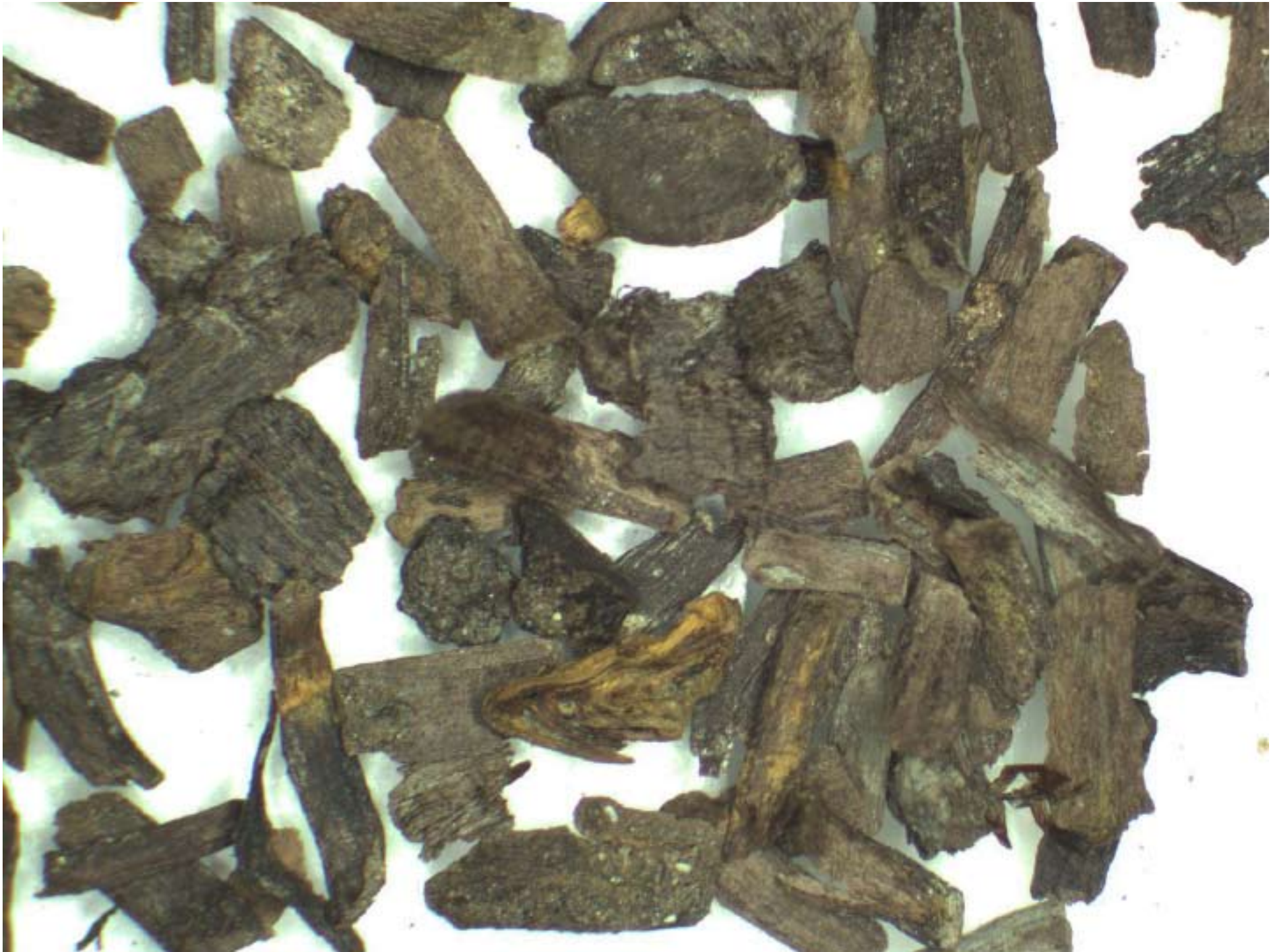
Figure 13. Sample 09DTSC11-M5 coarse ( >0.85 mm) fraction wood fragments. Note the 'flatness' and small size of the wood fragments as seen in all SC11 samples. For scale, the rounded fragment (top, center) is \sim 4 mm long.
