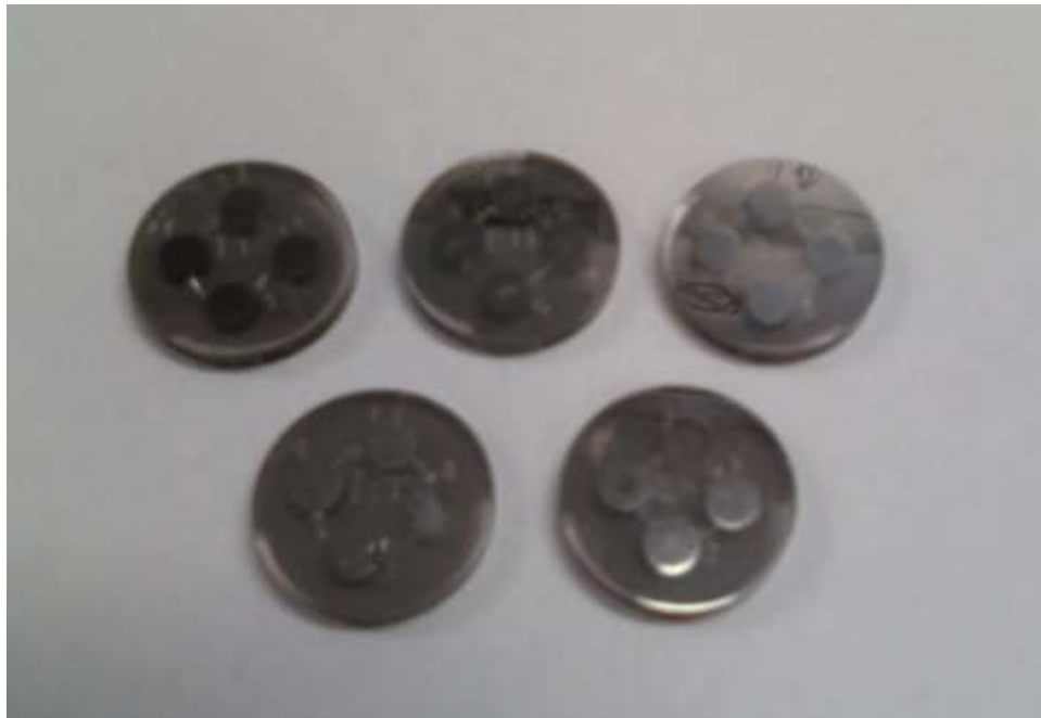
Figure 1.4. Acrylic disks with tephra samples for electron microprobe analysis. These disks have been coated in carbon.
