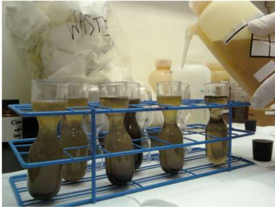
Figure 1.3. Separating the glass shards from the mineral content using tetrabromoethane. The glass has a lower density than the heavy mineral content. Darker samples typically have more organic material.
