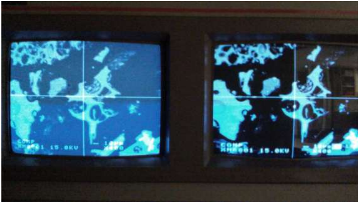
Figure 1.5. Electron backscatter images of glass shards using the JEOL electron microprobe at the University of Alberta.
