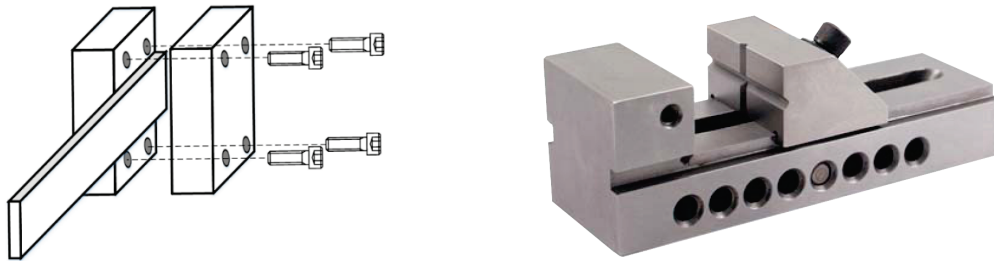
Figure 4-23: Early prototype clamp design (left) vs precision grinding vise (right)
