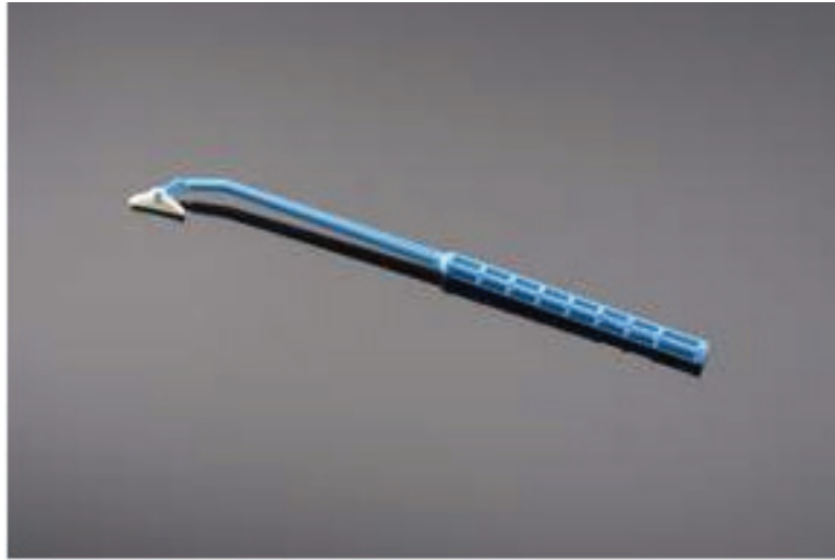
Figure 4.3 Photograph of a cell scraper from BD Falcon: 18 cm handle and 1.8 cm blade.
