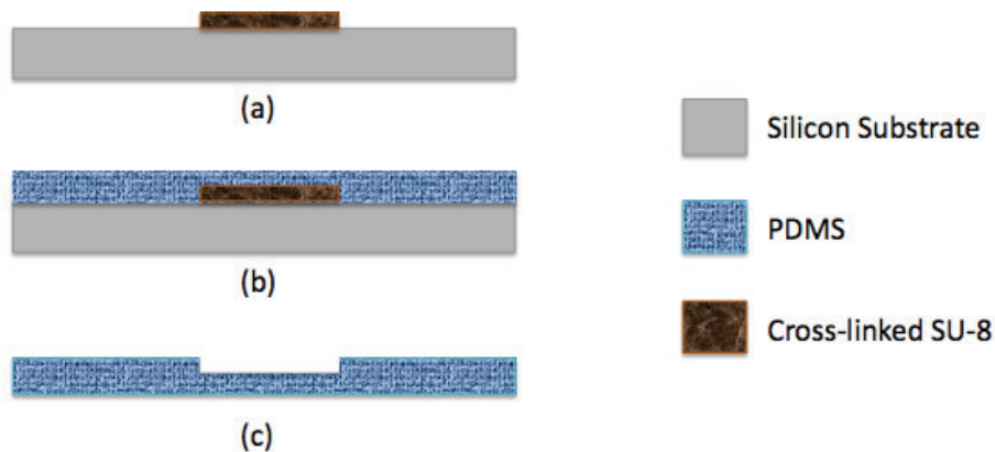
Figure 3.3 Fabrication process for PDMS fluidic and microfluidic channels: a) SU-8 mould fabricated using steps outlined in Figure 3.1; b) pour liquid PDMS onto the SU-8 mould; c) peel cured PDMS layer from substrate.
