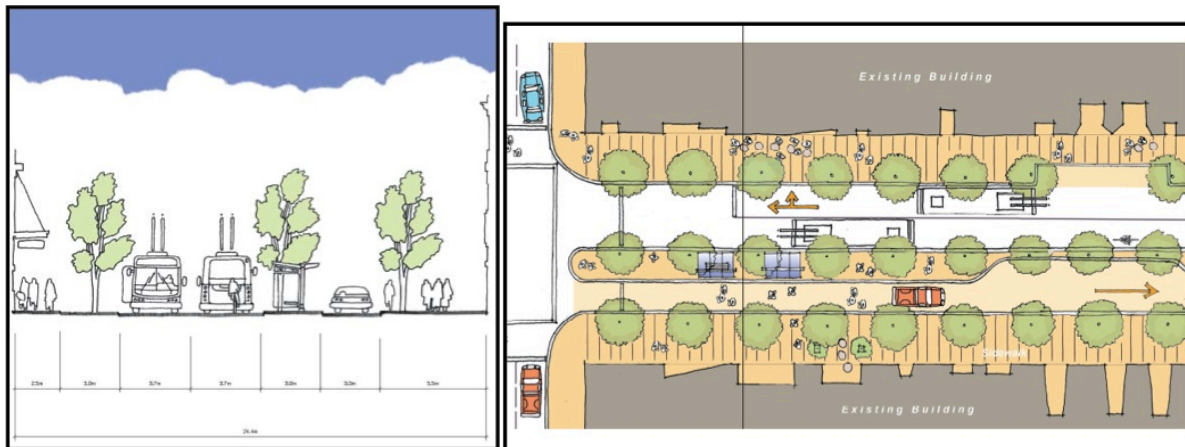
Figure 6: One Sided Flex and One Sided Flex North of Smithe (DV BIA) Concepts - Cross section and typical block plan views (Source: COV, 2006)
