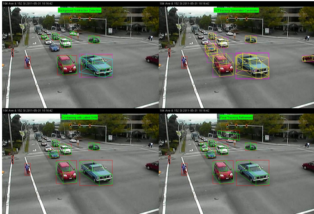
Figure 4.7: 3D localization results after background subtraction (top left), KLT tracking (top right), co-training (down left) and final refinement (down right).
