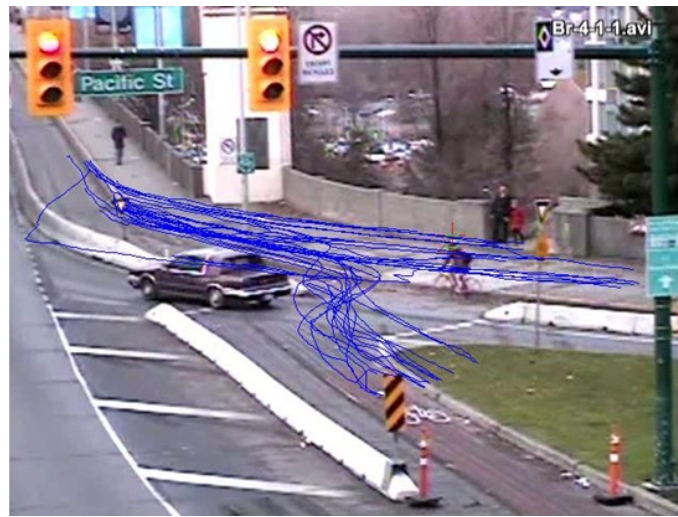
Figure 3.8: Burrard Bridge Northern Gate at Pacific Street. Blue lines show the tracks of the cyclists. Red \times indicates one example frame of the original track. Red + and the green box indicate the track of head.
