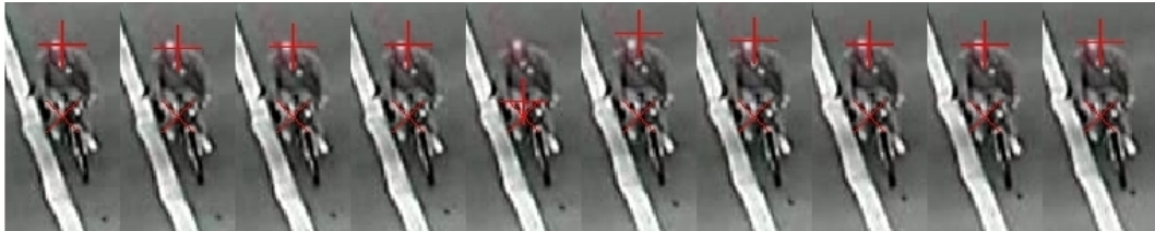
Figure 3.4: Ten consecutive frames from a video in the Surrey dataset. Red x indicates the original tracking point, red + indicates the location of the head. We are not able to move the tracking point to the top of the head in every frame.
