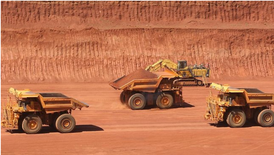
Figure 9: Robot Trucks Fitted with Radars, Lasers and GPS Systems
