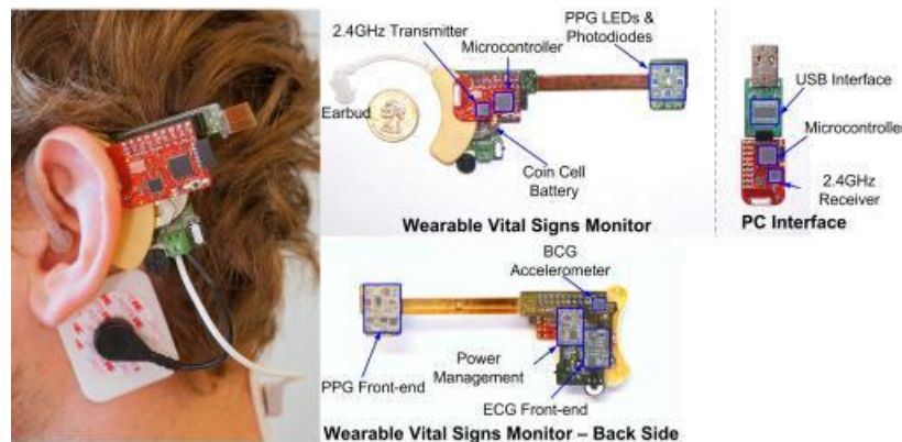
Figure 1-15 Left: The wearable vital signs monitor worn at the ear. Center: Front side and back side of the monitor. Right: PC interface. [84]
