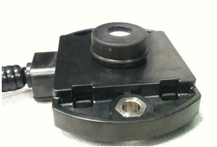
Figure 5 Sensor with RKI filter
