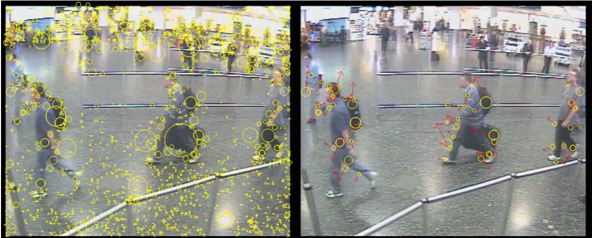
Figure 2.9: SIFT (left) and MoSIFT (right) interest points. Yellow circles indicate interest points and their scales, red arrows indicate the dominant motion orientation. Figure taken from [16].
