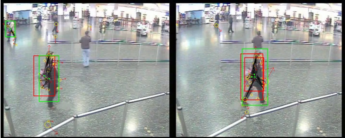
Figure 2.10: Detection process examples. Voting space (black lines), center hypotheses (green points), hypotheses (red rectangles) and final hypothesis (green rectangles). Figure taken from [16].
