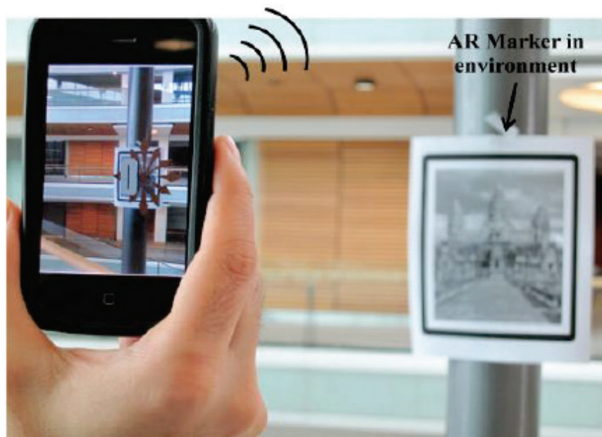
Figure 2.10. The user uses mobile devices to find “AR markers” in surrounding and obtain location information
