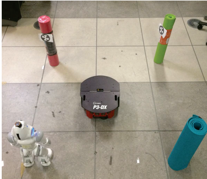
Figure 5.3. AR-EKF-SLAM experiment scenario. NAO walks to and observes landmark one by one and return to original location
