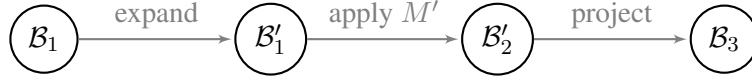
Figure 4.2: Module M := \pi_\tau(M') operates by (a) expanding vocabulary of input \mathcal{B}_1 , (b) applying M' to expanded input, and, (c) projecting the result of application of M' .
