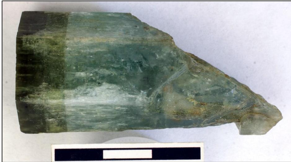
**Figure 4-4. Colour zonations parallel to the basal pinacoid from dark green (emerald) to light blue to colourless beryl. Sample from the Erongo deposit, Namibia. Scale bar in centimetres.**
