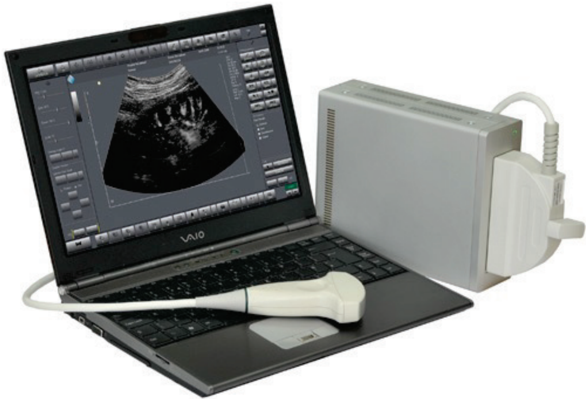
Echo Blaster 128 CEXT-1Z with attached transducer and notebook.
