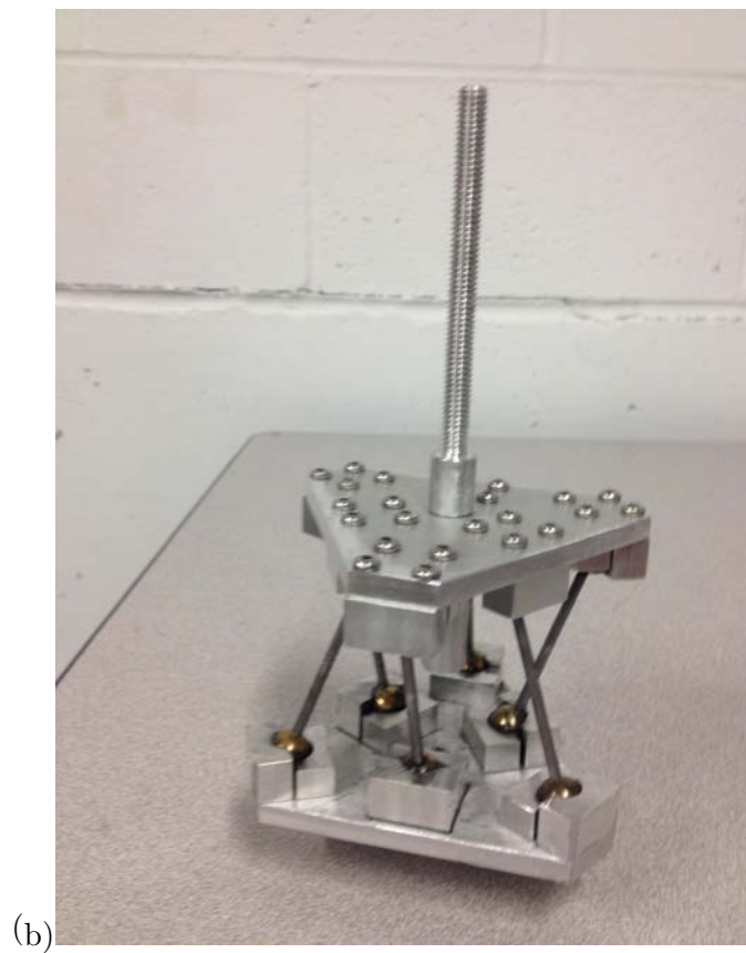
Figure 5.7: The algebraic screw: (a) Schematic diagram, (b) Developed prototype [149].
