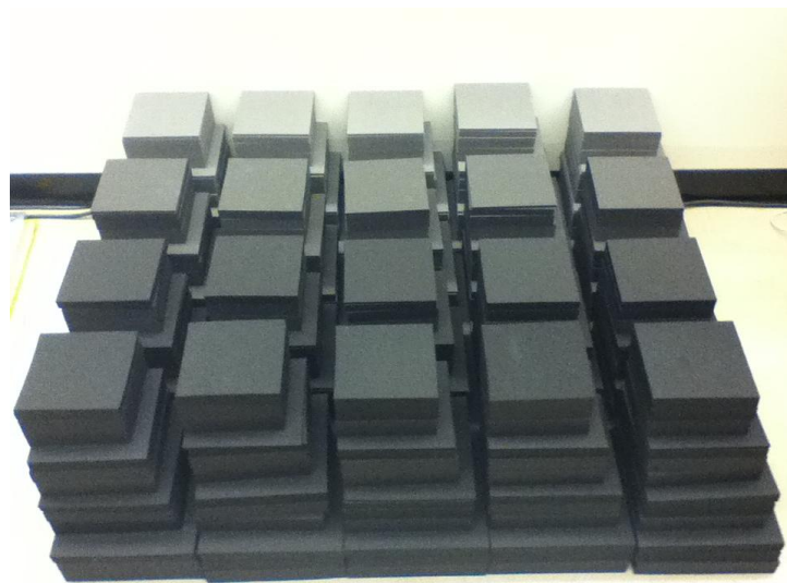
Figure 2-2. 64 Hip Protector Prototypes (5 samples of each) – Prior to Shaping
