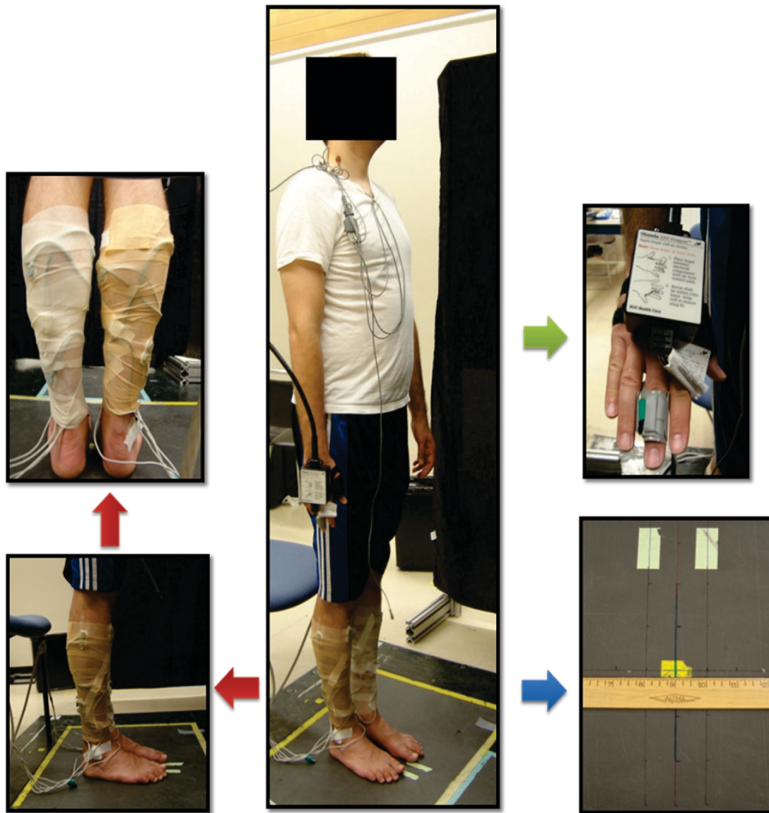
Figure 3-1 Quiet stance positioning and instrumentation: (Centre) Profile view. (Left) EMG electrode placement as seen from the rear and side view. (Right, top) BP finger cuff electrode attached to the middle finger of the participant. (Right, bottom) Heel positioning on force plate. A total distance of 5 cm between the toes of both feet.
